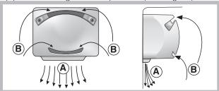
Pure Wind maximises air circulation, improving the efficiency of the evaporator and helping to achieve the optimal temperature inside the refrigerator as quickly as possible each time it has been opened. The blown air (A) is cooled when it comes into contact with the cold wall, whereas the hotter air (B) is sucked up (see diagram).
